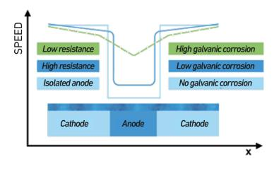
**The materials affected** Depending on the level of galvanic potential between them, the intensity of corrosion could be higher, reducing the useful life of the anodic material.
