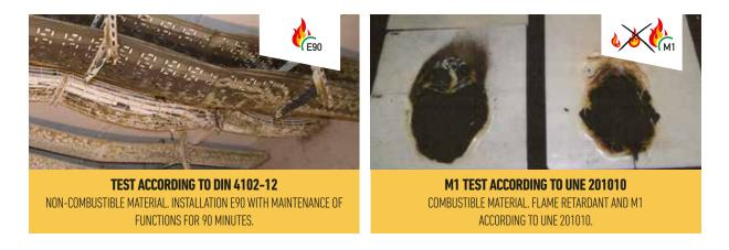
The market has tended to increase more and more the restrictions on non-flame propagating materials, so it has been necessary to use specific standards, of which the best known are the UNE 201010 on reaction to fire of electrical accessories (previously the UNE 23727 on construction materials was used) or the UL94 on flammability of plastic materials. The main classifications of these standards are as follows:
