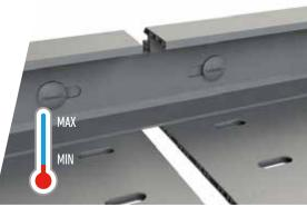
Our joining systems use longitudinal holes to absorb the movements due to thermal expansion. BASOR advises separating the straight sections leaving space for the joints to act as expansion joints and allow these movements. The length of the section of trays, the difference in service temperature and the material will determine the maximum length of straight section to install the joint as an expansion joint.
