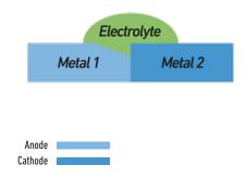
The one with the most negative reduction potential will be oxidized and the one with the most positive reduction potential will be reduced. It is important to bear in mind that for galvanic corrosion to occur, three conditions must be present simultaneously:
