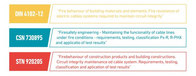
These standards define the test conditions to verify that the system, made up of fire-resistant trays, supports, accessories and cables, maintains electrical power for a specified time inside an oven in which the fire is simulated following a defined temperature-time curve.
