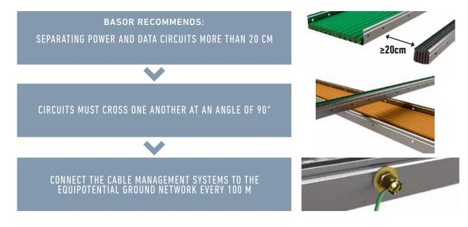
In situations where space is limited, different circuits can be installed in the same CMS dividing by means of a metallic separator. With correct installation that guarantees electrical continuity, it is NOT necessary to include a copper wire throughout the entire tray.
