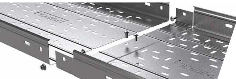
Impedance at the junction between pieces less than 50 mΩ
