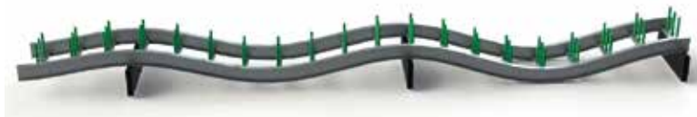
Determination of SWL in multi-span (IEC 61537)
